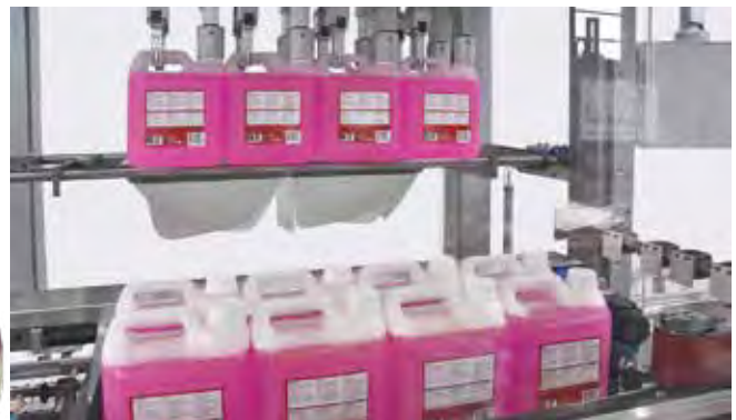
Packing of canisters with layer grouping device.
