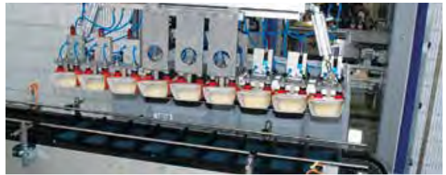
Packing of pouches with collating unit in a dual flighted chain.
