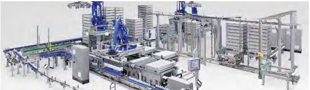
Total system for autoclaves loading / unloading in the pharmaceutical industry.
