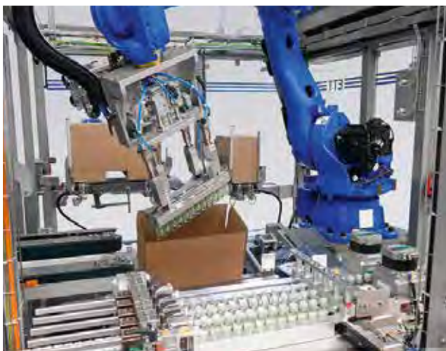
Case magazine (in the background) and product collating unit (at the forefront) with robot handling head.
