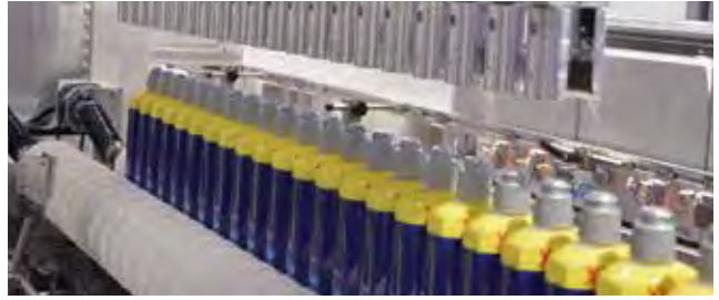
Packing of bottles with flowing lifting movement out of the screw collating unit.
