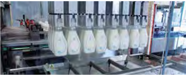
Universal gripper head for depositing products into several cases at a time.
