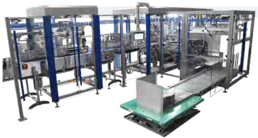
Continuously high speed wraparound machine WP 40-3. Intermittent wraparound machine WP 30-2 with automatic magazine equipping.
